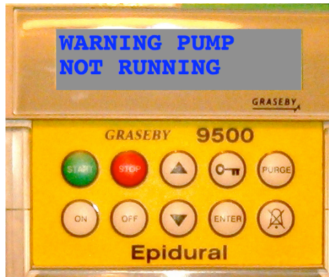
Fig. 1. Partial screen shot of the simulation—a user can mouse click on the buttons, which are animated to give simple visual feedback of pressing. Note that graph theory does not address all HCI issues, such as the naming or confusibility of buttons.
