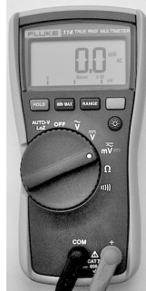
Fig 1. The Fluke 114, showing the LCD, five buttons and the knob. Two test leads are plugged into the bottom of the device. The device is 75×165mm — easily held in one hand.
