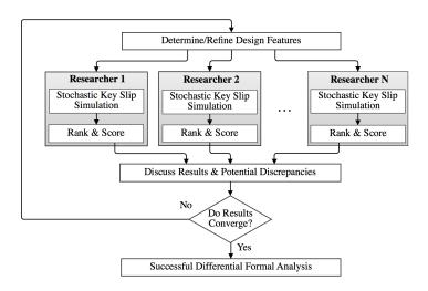
Figure 3: The Differential Formal Analysis Process
