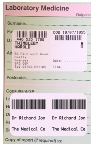
Figure 2: A very simple bug to see, with preventable consequences. The computer-printed label has unnecessarily truncated the doctor’s name and where he works, though it had no problem with the patient’s long surname. The doctor’s surname is not Jon, and he does not work in a Medical Ce! If a name has to be truncated, it should be displayed as “Dr Richard Jon. . .” making it clear something is missing, or the first name could have been abbreviated, perhaps down to an initial (which is conventional practice). One day, items labelled incorrectly will be misplaced or used with the wrong patients.
